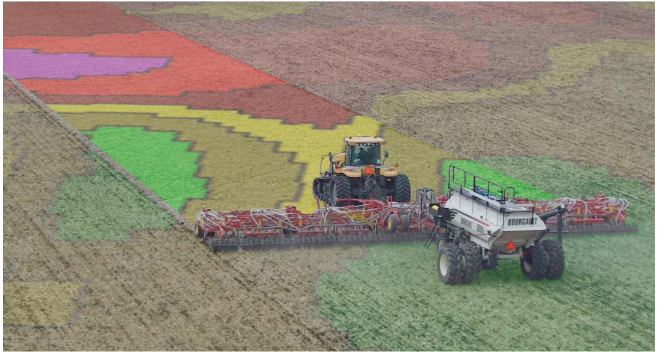
This map overlay shows the zones of a field as they are seeded using global positioning systems.
